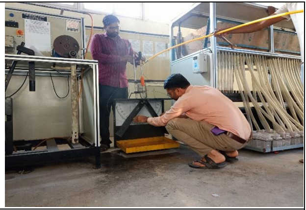
Spray angle measurements of Sprayer
