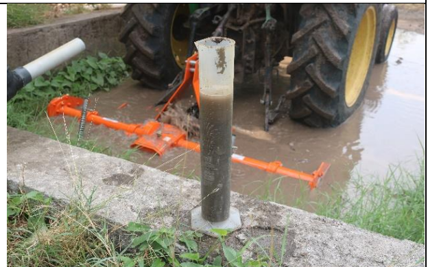
Testing of rotavator water puddling
