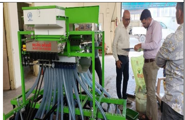
Laboratory testing of multi crop seed cum fertilizer drill
